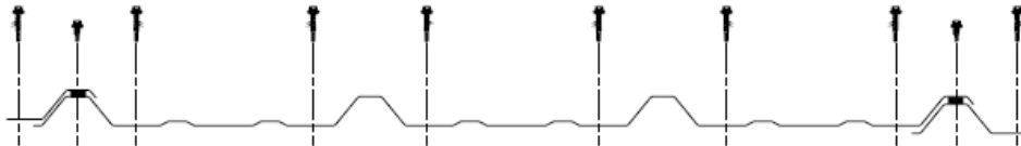
PBR-Panel Fastening Pattern - Ends
