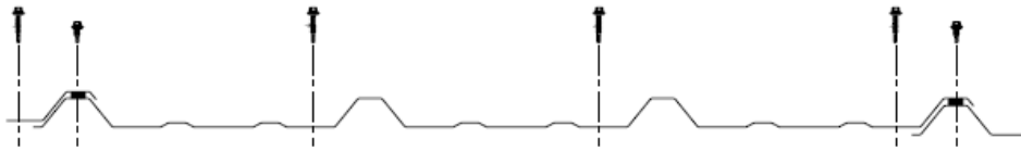
PBR-Panel Fastening Pattern - Interior
